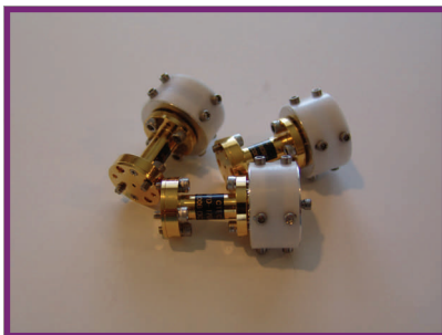
170 GHz Omni-directional Antenna
