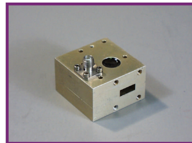
Circulator with Coax Adapter
